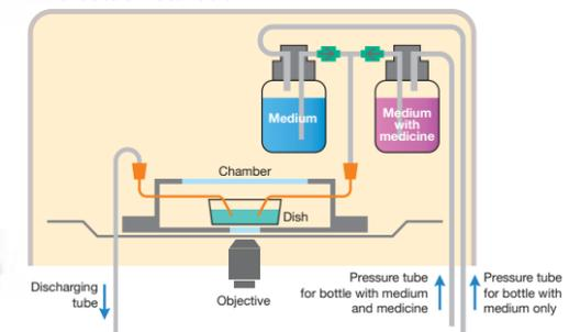
\*Syringe pump or peristaltic pump is necessary to pressurize the solution bottles.
