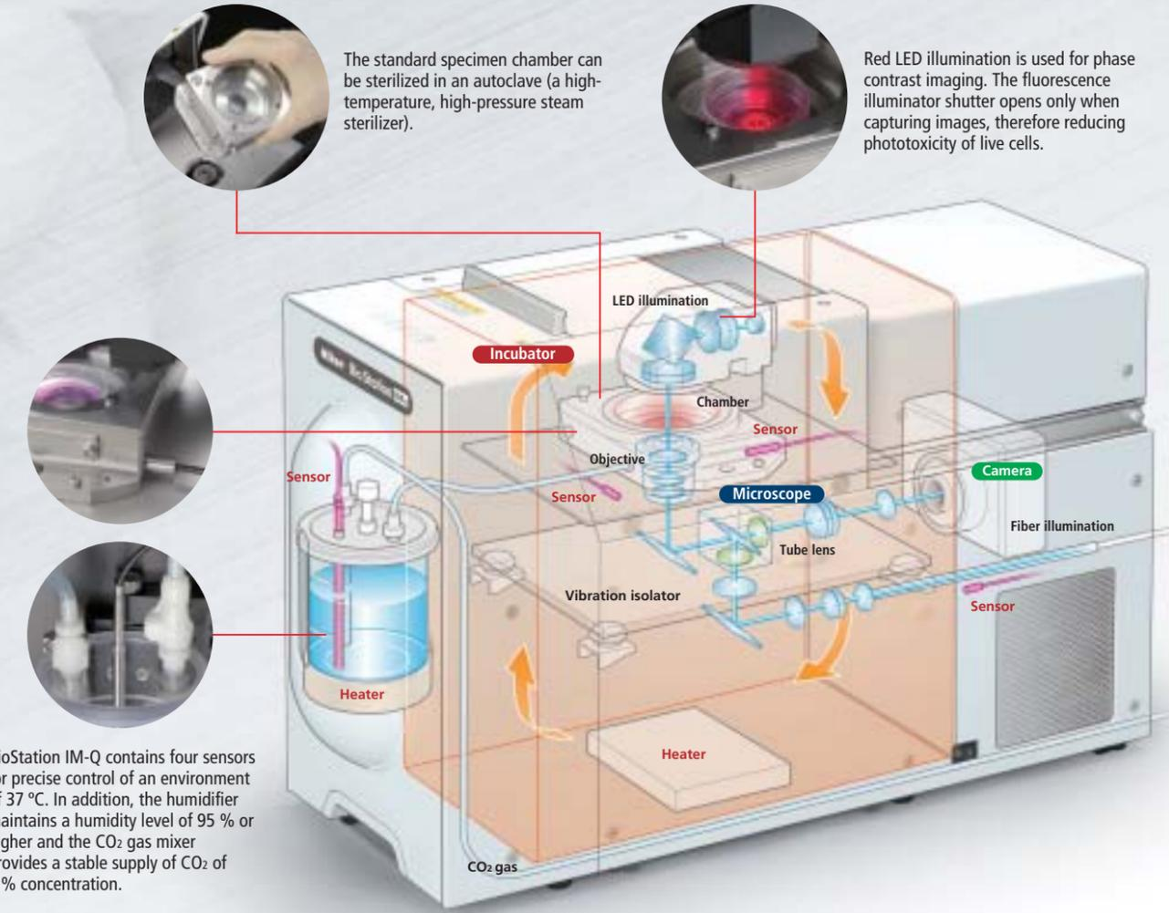
BioStation IM-Q contains four sensors for precise control of an environment of 37 °C. In addition, the humidifier maintains a humidity level of 95 % or higher and the CO<sub>2</sub> gas mixer provides a stable supply of CO<sub>2</sub> of 5 % concentration.
