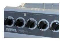
Individually control the precise, variable dosing of suspensions and lubricants with two second to five minute dosing intervals
