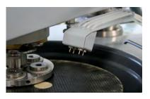
Exact droplet dosing with reverse rinsing function keeps lines clear and ready for use
