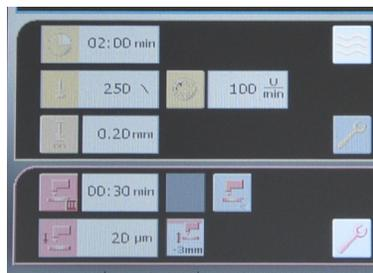
**Graphical Touch Screen Control Panel** provides complete process control and programmability, including the ability to save and password protect procedures
