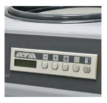
Sealed **Touch Button Controls** for water, speed and disc cooling
