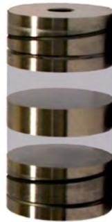
Unique **Cylinder** design prevents seizure by allowing out-gassing during resin melt. Intermediate ram allows the **Opal 460** to produce two mounts per cycle
