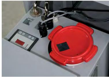
Optional **Recirculation Coolant System** maintains constant water temperature with refrigeration coils
