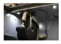
**LED illumination** bathes the cutting chamber in a cool white light and is neatly incorporated in the design of the chamber to allow for unencumbered operation
